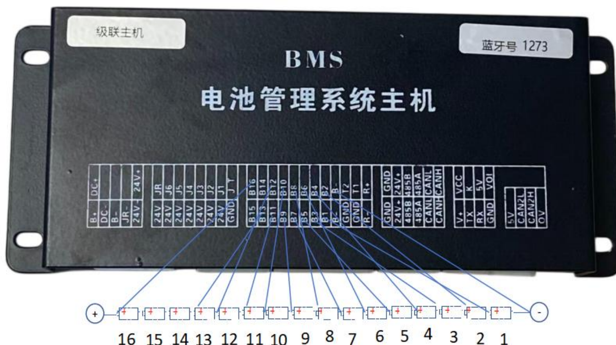
Wiring Diagram of Master BMS VS 14 CELLS 14串接线图
