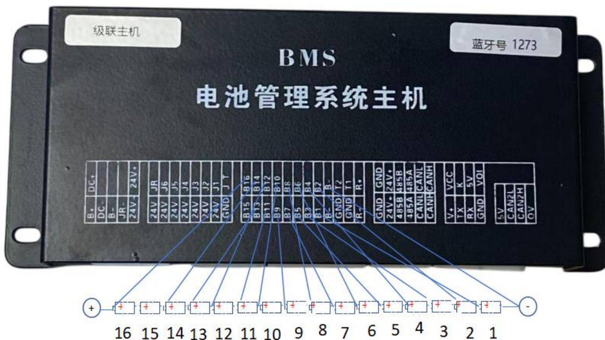
Wiring Diagram of Master BMS VS 15 CELLS 15串接线图
