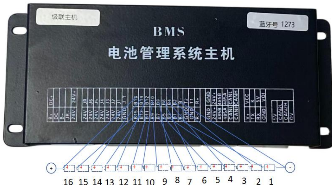
Wiring Diagram of Master BMS VS 16 CELLS 16串接线图
